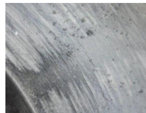
Fig.7 Natural grinding burn
