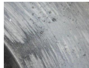
Fig.7 Natural grinding burn
