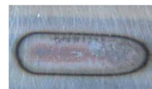
Fig.8 Artificial laser grinding burn
