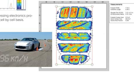
With 65,536 sensing points sampled at 450 fps, the HS Tire System generates high resolution images and accurate tire interface pressure data at speeds up to 140 km/h.
