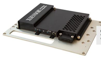
Data logger records data from up to four sensor packs and up to a total 256 x 256 sensing array.
