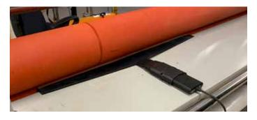
Ensure proper balance and calibration between your rollers to prevent misalignment of your equipment or product damage. The Nip Roller Pressure System was designed for companies and manufacturers that rely on accuracy and repeatability of their own machines. XSENSOR's Nip Roller Pressure System provides quantifiable, unbiased data and visualizations that help get your machines properly aligned, balanced, and calibrated.
