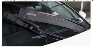
repeatable and sensitive line load sensor giving the wiper blade line load a profile on the windshield. The PX100:10.160.05 wiper blade sensor provides more sensing points than XSENSOR's previous models, and an improved design which makes the sensor more repeatable and accurate to line load estimations. The sensing area is 25.4mm x 812.8mm, allowing for measurements of car, truck, and aviation wiper blades.
