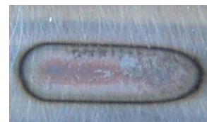
Fig.8 Artificial laser grinding burn
