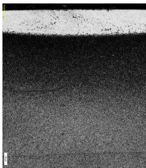
Fig.11 600W laser, re-hardening zone (230 \mu\text{m} )
