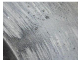
Fig.7 Natural grinding burn
